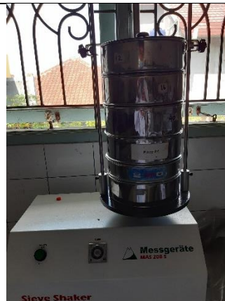
Alat : Sieve Shaker Mesh : 12, 16, 40, 44, 100
